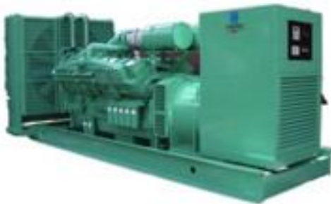
1000 KVA / 800 KW Cummins KTA38 G2 220 - 480 V 60 Hz Lubrication: 120 liters Fuel at Load: 0.204 L/kWh
