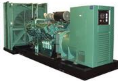
1160 KVA / 928 KW Cummins KTA38 G5 220 - 480 V 60 Hz Lubrication: 135 Liters Fuel at Load: 0.222 L/kWh
